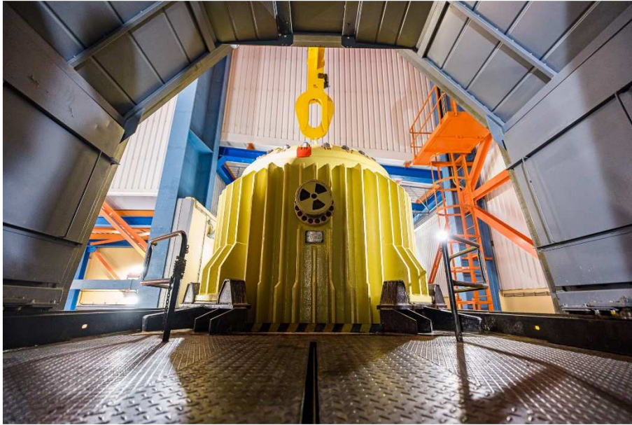
Figure 1.3.4-2: Transport cask being on railway carriage in the KKÁT
