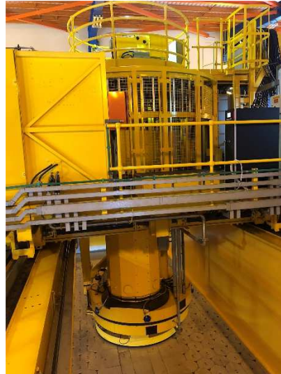
Figure 2.4.3.-2: Tower of KKÁT facility refuelling machine. The 12 angled metal cover, under which the Jabroc 'N' beechwood is located, can be seen at the lower part.
